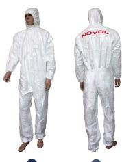
White coating overalls made of Tyvek of a fabric weight  $42g/m^2$ . Protect from dust and liquid particles (they provide protection compliant with the  $3^{rd}$  category of protective clothing, Type 5- dust-proof, Type 6- a limited spraying tightness). They are durable and resistant to tearing and frays as well as being antielectrostatic and comfortable. Tyvek is waterproof but it lets air and steam permeate.
