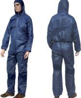
Blue protective overalls made of polypropylene nonwoven fabric of  $40g/m^2$ , which, considering their lightness, provide sufficient mechanical resistance. They efficiently protect against dirt, do not cause overheating or perspiring, whilst providing a high level of comfort. Sufficient protection from dust  $> 5 \, \mu$ m.
