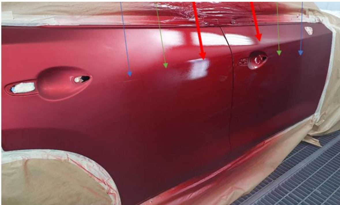
3. Third layer of tinted clearcoat
