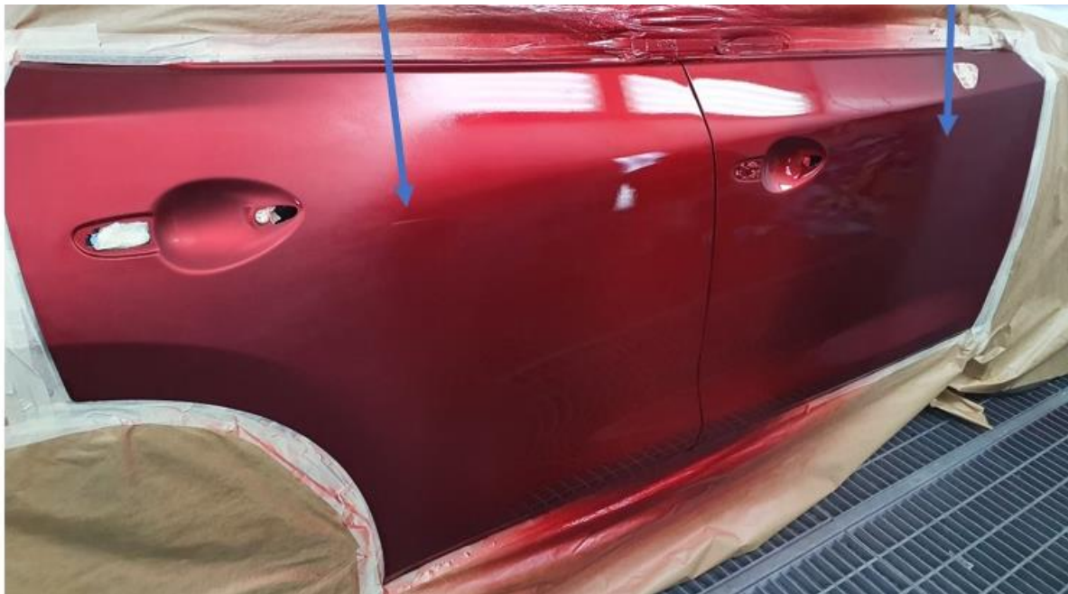
1. First coat of tinted clearcoat
