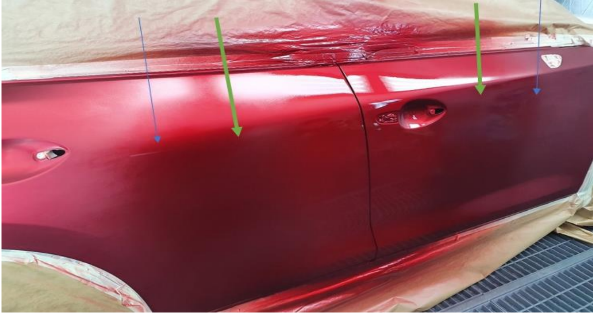
2. Second layer of tinted clearcoat
