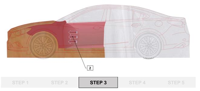
$\rightarrow$  1 Apply the drop layer on the part to be recoated.
